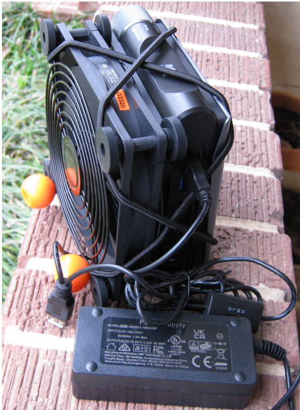
Figure 1: The AMR5 Mini PC with its power supply, and a case fan attached with bungee cords.
